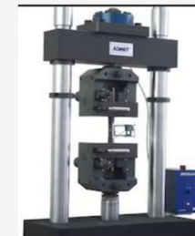
Tensile Strength and Bend Test on Reinforcement
