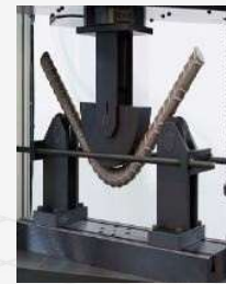
Tensile Strength and Bend Test on Reinforcement
